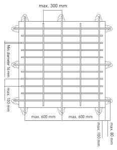
Recommended measurements for window bars
