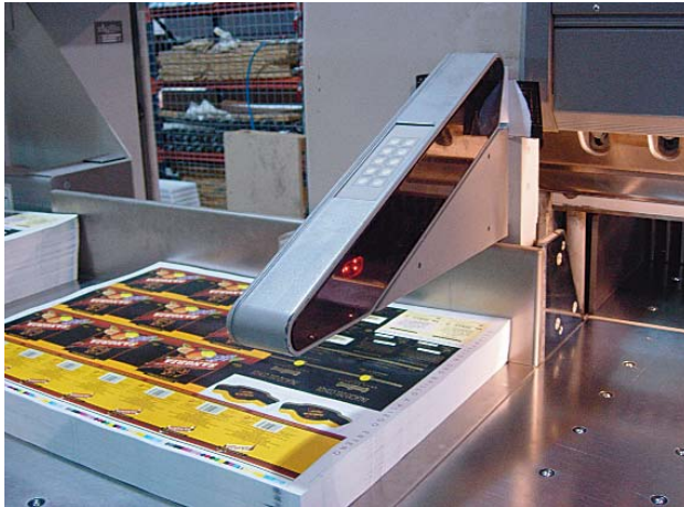
Paper guillotine fitted with photoelectric cells as a safety measure
