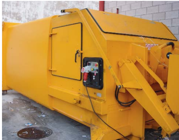
Waste paper compacter
