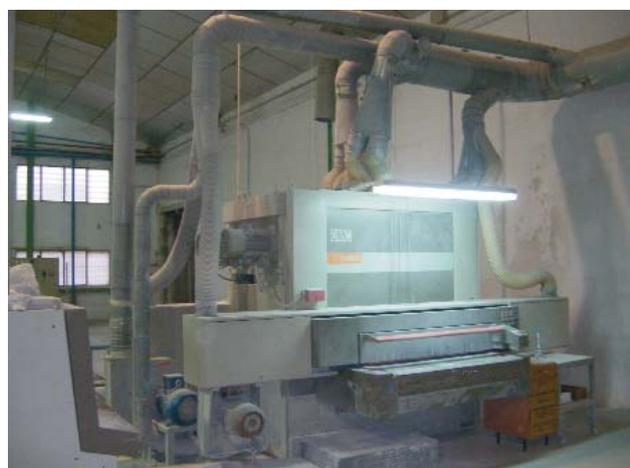
Sanding machine with vacuuming system
